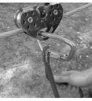
mantle of the rope on a length of 2 meters. Fortunately, the core of the rope was not damaged. After lowering the participant by a few meters, the carabiner jumped back into the normal position. No one suffered any physical injuries.
