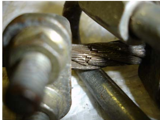
Picture 2: Example of equipment located between two wire rope grips
