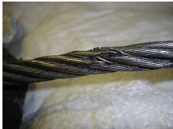
Picture 1: A typical break on a zip wire or belay cable
