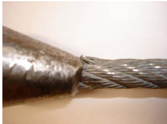
Picture 3: Example of cable able to rotate / bend about a fixed point
